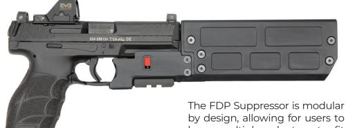
By attaching to the pistol's frame, the FDP suppressor does NOT require a threaded barrel, nor a Nielsen Device/Booster assembly. The patented attachment system does not require a booster adapter since the host pistol operation is not changed. This also maximizes ammunition compatibility, allowing supersonic and subsonic loads to be used.
